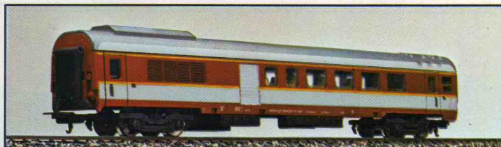
30 9311 French composite 1st class/luggage coach «Grand Confort», series A4Dtux, of the S.N.C.F. - Length 268 mm.
